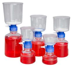
Thermo Scientific<sup>™</sup> Nalgene<sup>™</sup> Rapid-Flow<sup>™</sup> Sterile Disposable Filter Units and Disposable Bottle Top Filters are designed with a unique membrane support plate that's welded into its housing to help ensure membrane fluid path integrety.
